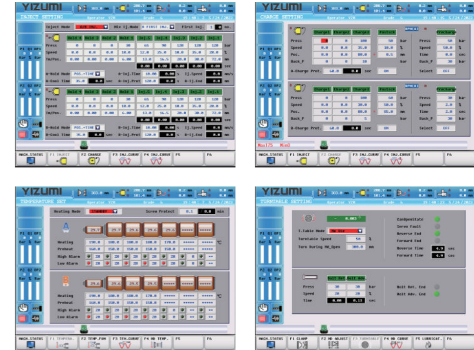
Interface of dedicated industrial controller ▲
